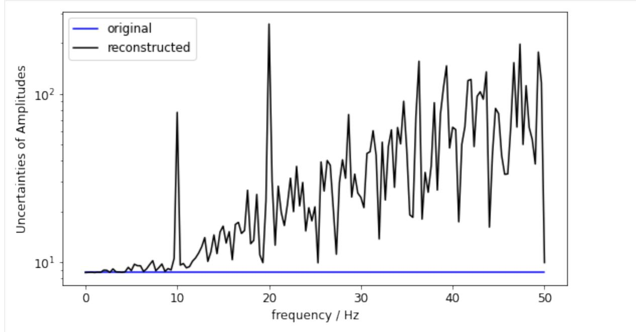
Note: We just divided by the lowpass' transfer function. To readers with some background in control theory it should be obvious that this amplifies high frequencies and might lead to instabilities if used inside a control loop. However, because we are taking the signal's and filter's uncertainty into account, the reconstructed spectrum shows us just that - *that the higher spectrum values are much more uncertain*.
