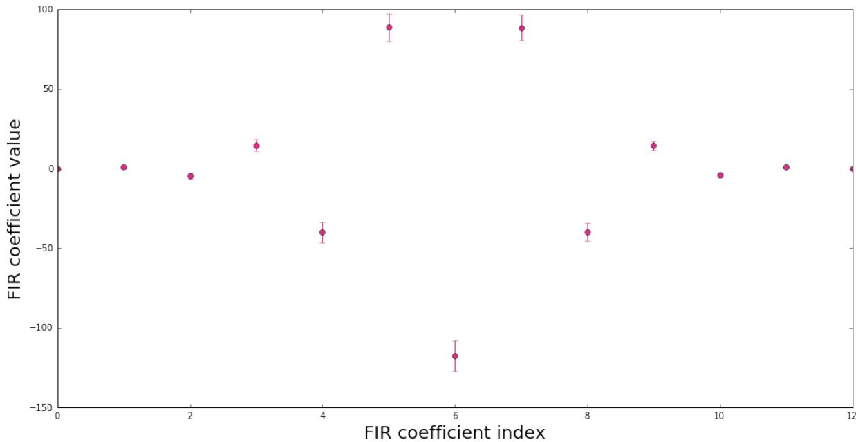
In order to render the ill-posed estimation problem stable, the FIR inverse filter is accompanied with an FIR low-pass filter.
