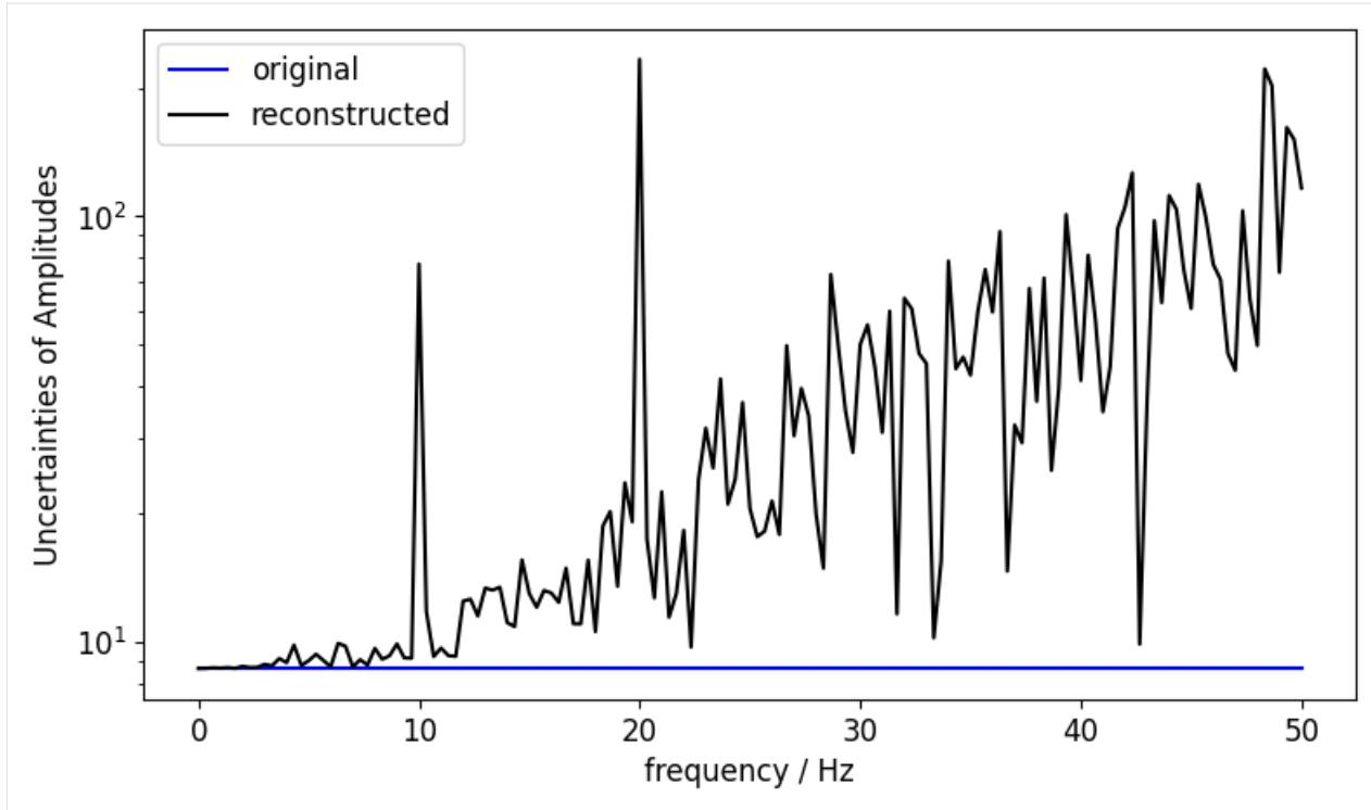
Note: We just divided by the lowpass' transfer function. To readers with some background in control theory it should be obvious that this amplifies high frequencies and might lead to instabilities if used inside a control loop. However, because we are taking the signal's and filter's uncertainty into account, the reconstructed spectrum shows us just that - *that the higher spectrum values are much more uncertain.*
