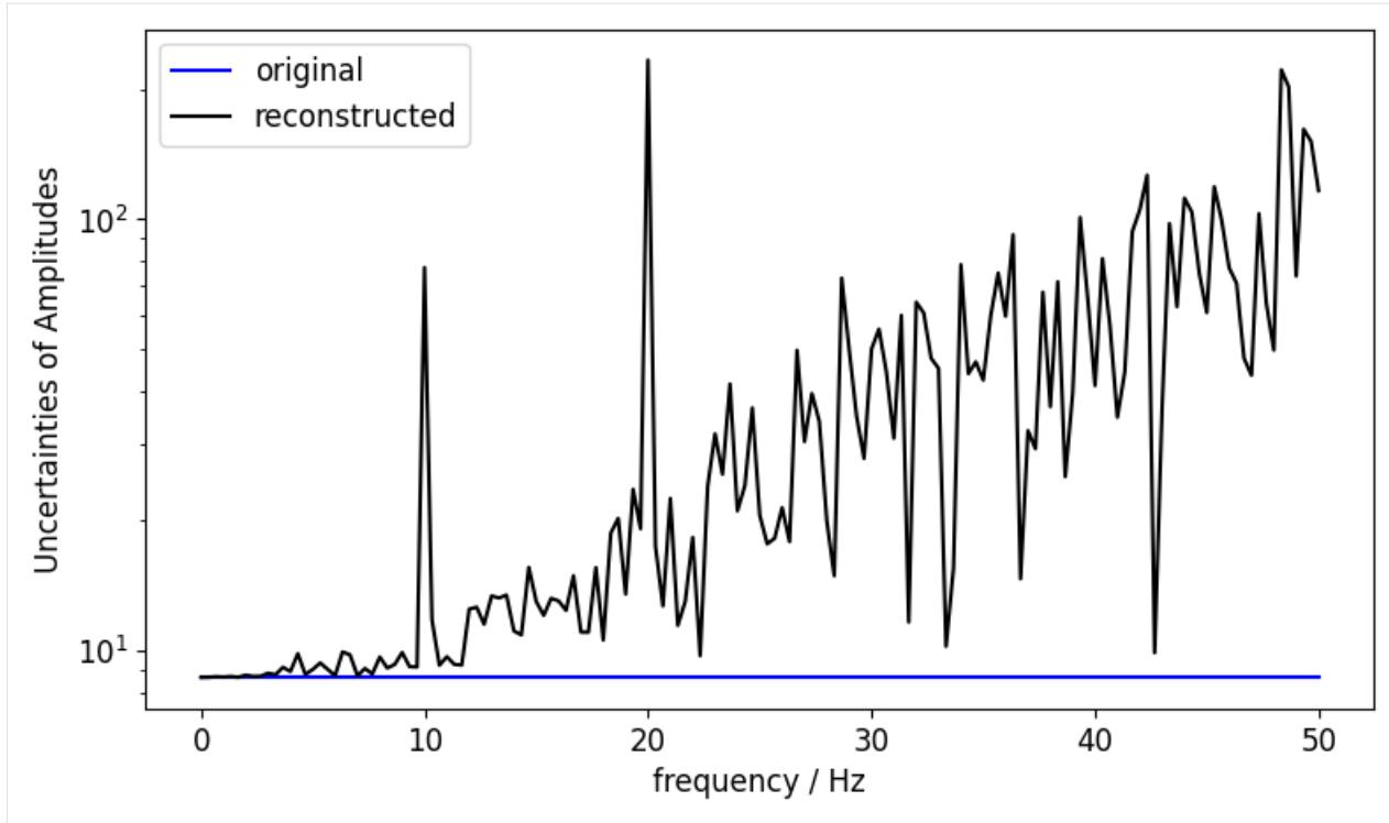
Note: We just divided by the lowpass' transfer function. To readers with some background in control theory it should be obvious that this amplifies high frequencies and might lead to instabilities if used inside a control loop. However, because we are taking the signal's and filter's uncertainty into account, the reconstructed spectrum shows us just that - *that the higher spectrum values are much more uncertain.*
